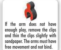
If the arm does not have enough play, remove the clips and thin the clips slightly with sandpaper. The arms must have free movement and not bind.
